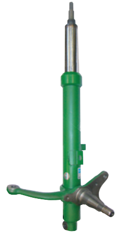
Komplettes Achsbein Complete suspension 35-003922 (Porsche 911)
